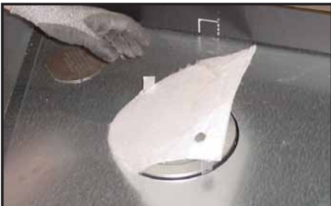
Figure 9.2 Remove the white gasket material covering the seal cap.
