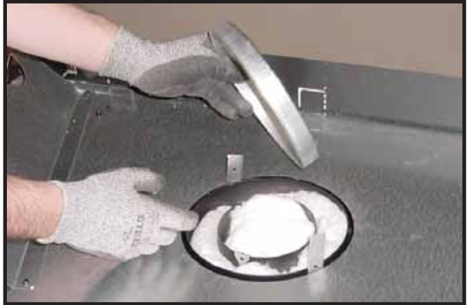
Figure 9.3 Remove the seal cap.
