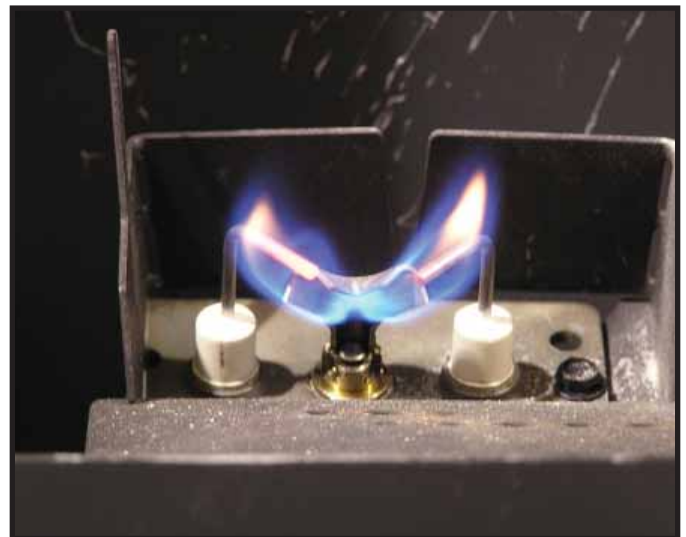
Figure 3.1 IPI Pilot Flame Patterns
