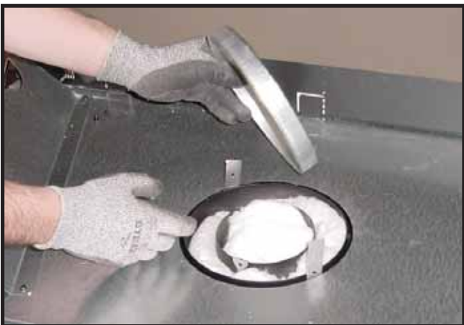
Figure 9.3 Remove the seal cap.
