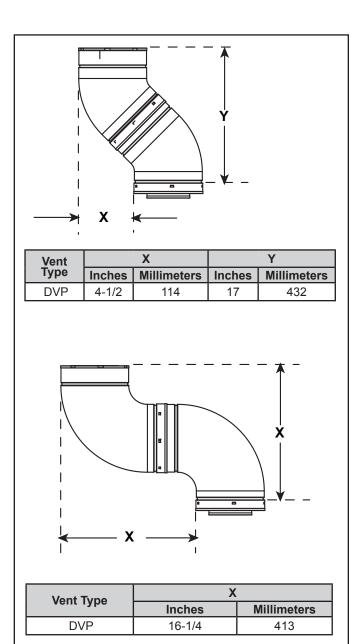
Figure 4.5 Vertical and Horizontal Offset for DVP Elbows
