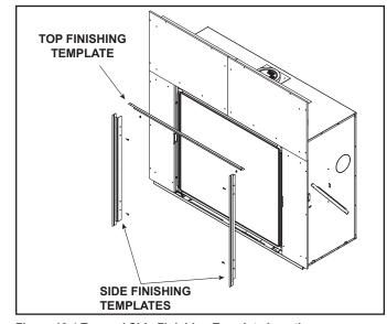
Figure 10.4 Top and Side Finishing Template Locations
