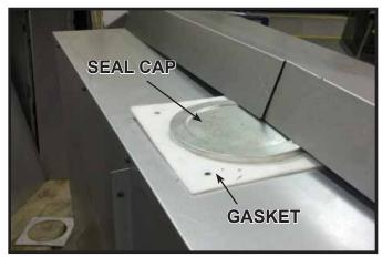
Figure 6.2 Seal Cap and Gasket Location
