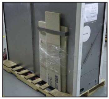
Figure 6.6 Shipping Location of Non-Combustible Board
