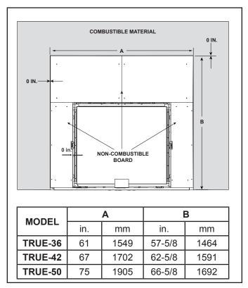
Figure 10.1 Non-combustible Facing Diagram
