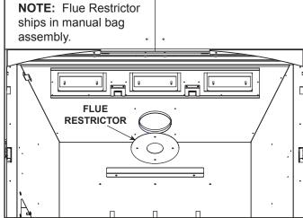
Figure 4.10 Flue Restrictor Installation
