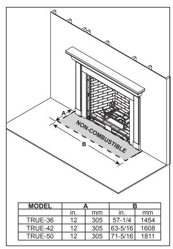
Figure 3.9 Non-Combustible Hearth Extension Dimensions
