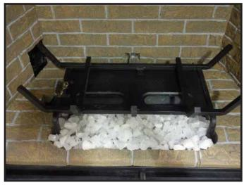
Figure 11.9. Ember Glass Area Covered with Teco-Sil
