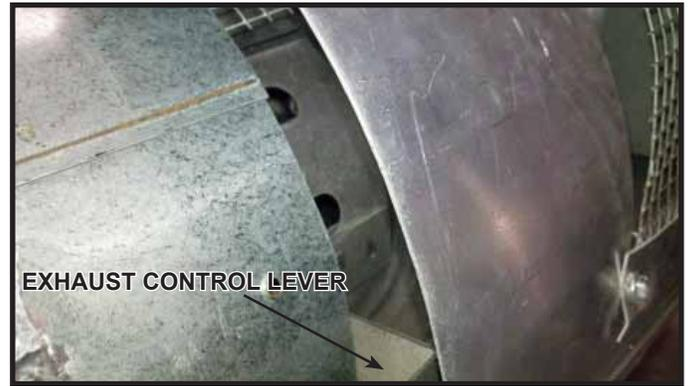
Figure 4.12 PVK-80 Control Lever Adjustment - Open
