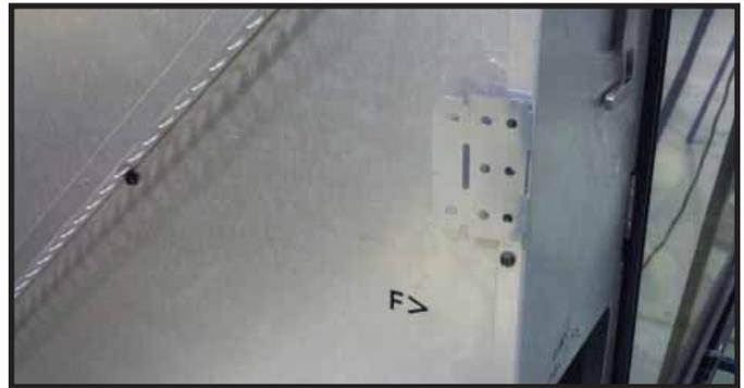
Figure 6.3 Side Nailing Tab in Shipping Position
