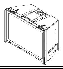
This appliance may be installed as an OEM installation in manufactured home (USA only) or mobile home and must be installed in accordance with the manufacturer's instructions and the Manufactured Home Construction and Safety Standard, Title 24 CFR, Part 3280 in the United States, or the Standard for Installation in Mobile Homes, CAN/CSA Z240 MH Series, in Canada.
