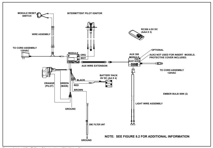
Figure 8.1 Intellifire™ Plus Pilot Ignition (IPI) Wiring Diagram
