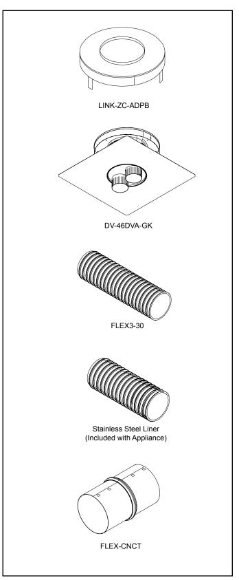
Figure 12.2 Direct Vent Flex Liner Accessory Kits
