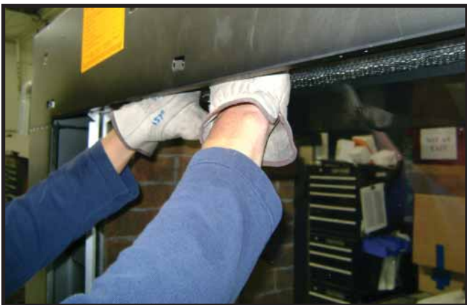
Figure 14.6 Top Glass Latch Access
