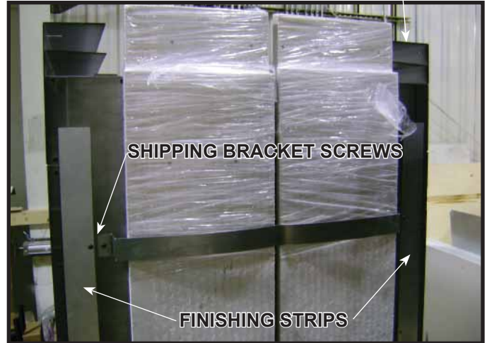
Figure 9.3 Shipping Brackets and Finishing Strip Locations.
