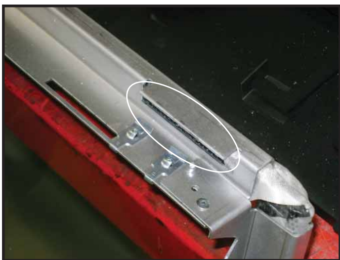
Figure 14.1 Glass Top Tab Detail.
