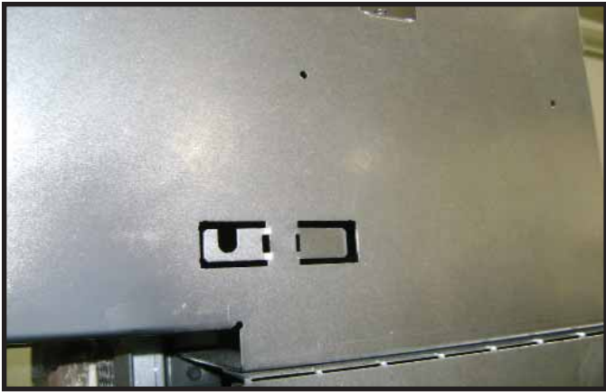
Figure 14.28 Mesh Rod Support Tabs
