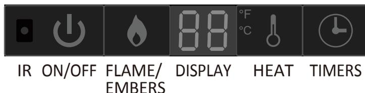
**a. IR:** Receiving infra-red signals(inputs)
