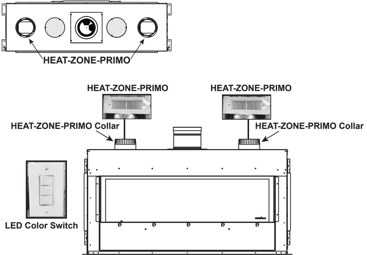
Figure 10. HEAT-ZONE-PRIMO Configuration
