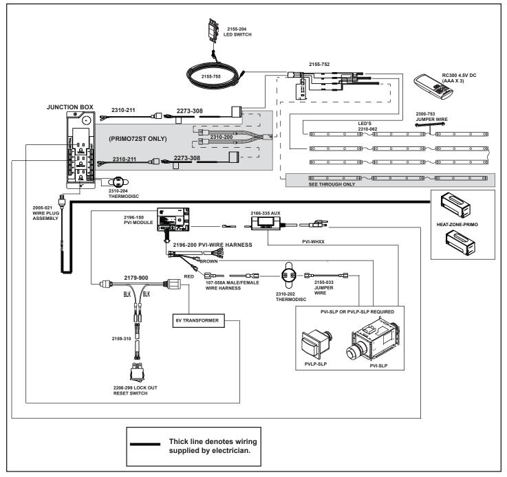
Figure 11. HEAT-ZONE-PRIMO Wiring Diagram
