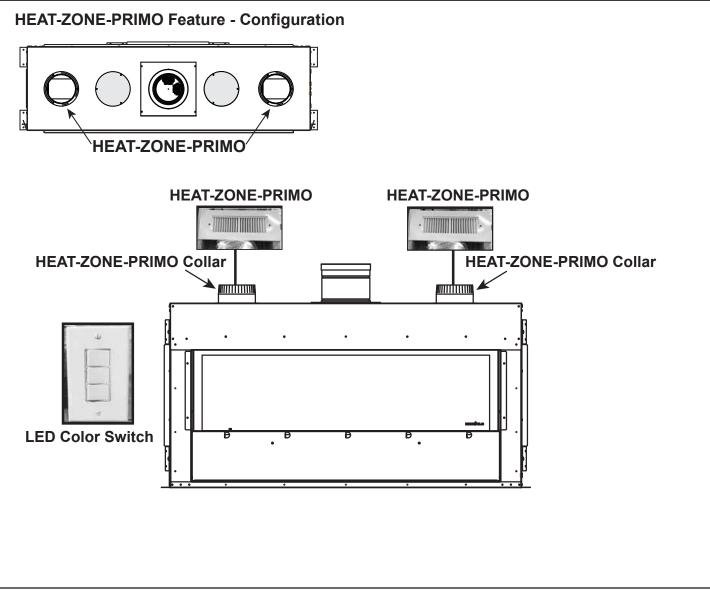
Figure 10. HEAT-ZONE-PRIMO Configuration
