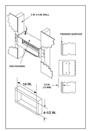
Figure 7. Wall Mounting (2 X 4)
