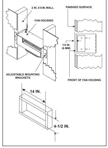
Figure 6. Wall Mounting (2 X 6)
