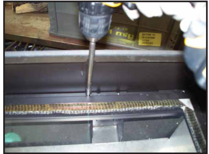
Figure 9.4. Gas and Electrical Access - Remove Glass Window
