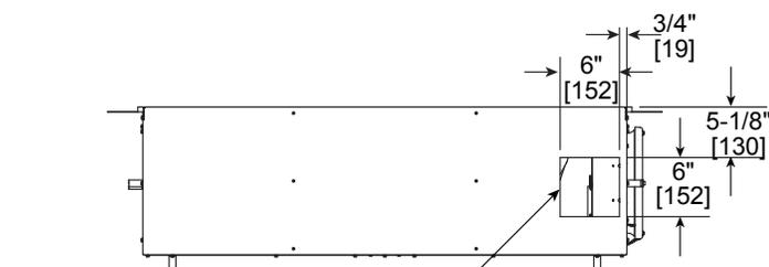
Gas access location on appliance if control box is located on side of appliance
