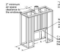
\* Framing must be filled in to top of front stand off after unit is installed.
