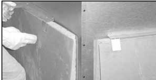
Figure 3.5 Unpacking Back Refractory
