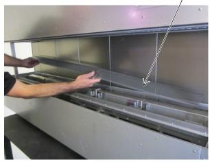
Remove the burner lock-down bracket (it is held in place with a single screw). .
