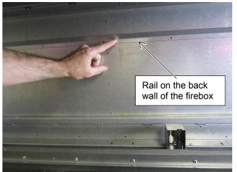
Install each fireback using suction cups (or two hands). Place the fireback into position, making sure the notch fits over the rail. Once attached, the fireback may be slid left or right. Once all firebacks are installed, make sure they are equally spaced and fully seated.
