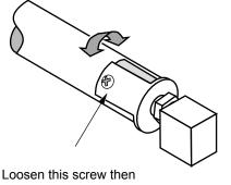
rotate the air shutter to adjust the air shutter.
