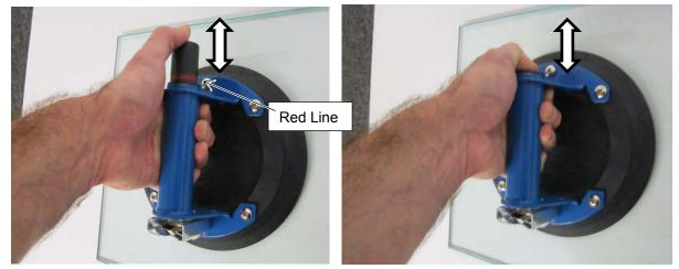
(b) Repeat step "a" for the remaining suction cups. NOTE: The suction cups have a lever opposite the suction button. This lever releases air, allowing the suction cup to disengage from the glass. <u>DO</u> NOT PRESS THIS LEVER UNLESS YOU ARE RELEASING THE SUCTION CUP.
