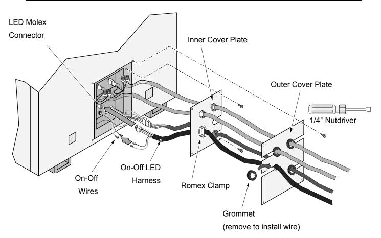
• The opposite end of the On-Off LED harness attaches to the on-off switch and LED controller (see "Installing the On-Off Switch and LED Controller" on the following page for details).
