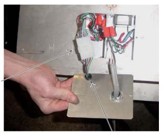
Use pliers to compress the strain relief from the top and bottom while pushing it into the hole in the bracket.
