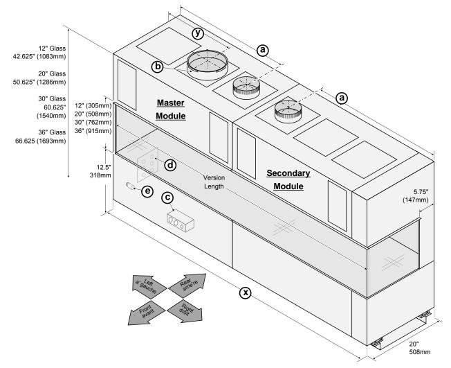
**NOTE**: The master module is always on the end that has a steel end.
