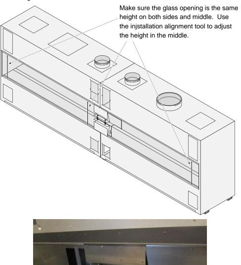
To align the glass opening, place the alignment tool between the two modules. Use the wing nuts to expand the support until it is tight. Measure the glass opening height on one side. Then measure where the two modules come together. This height should be identical. Use the wing nuts to expand the support as needed until the glass opening height is uniform. Do not remove the alignment tool until the Titan Lock connectors are fully tightened (see next page).
