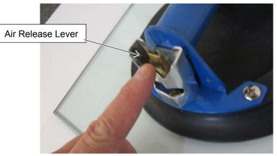
(c) Verify the suction cups are properly aligned and the red line is submerged before lifting the glass (see photos below).
