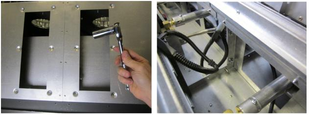
**NOTE**: After tightening the Titan Locks, double-check the glass opening height. It should be uniform across the width of the glass opening. If it is not, you will need to loosen the titan locks, adjust the alignment tool, then re-tighten the titan locks.
