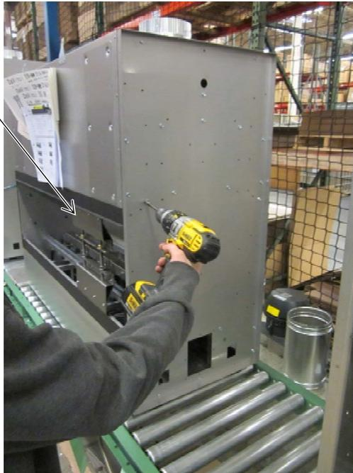
***Remove Components to Allow for Fireplace Joining*****Remove Media Trays and Burners Near Center of Fireplace**
