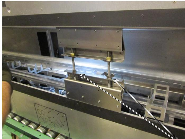
To align the glass opening, place the alignment tool between the two modules. Use the wing nuts to expand the support until it is tight. Measure the glass opening height on one side. Then measure where the two modules come together. This height should be identical. Use the wing nuts to expand the support as needed until the glass opening height is uniform. Do not remove the alignment tool until the Titan Lock connectors are fully tightened (see next page).
