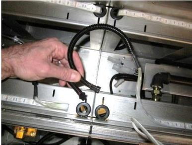
**After Titan Locks are Installed, Route LED Wires Through the Grommets Access Holes**
