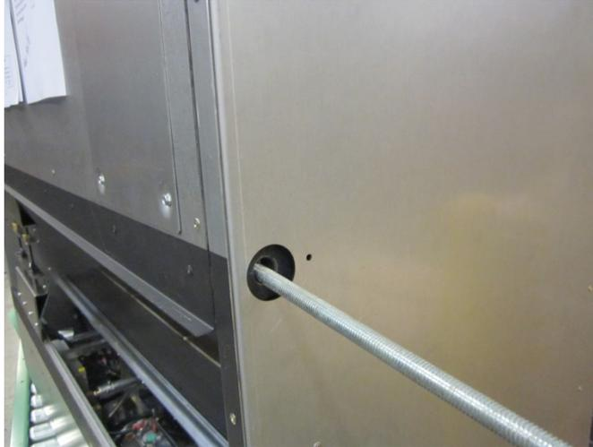
**NOTE:** Do not tighten the tension rods until the titan connectors are in place and the glass opening is aligned – see “Order of Intallation”.
