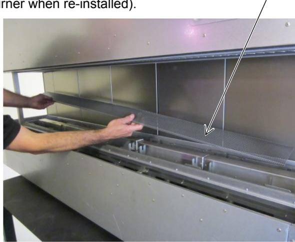
Remove the burner lock-down bracket (it is held in place with a single screw).
