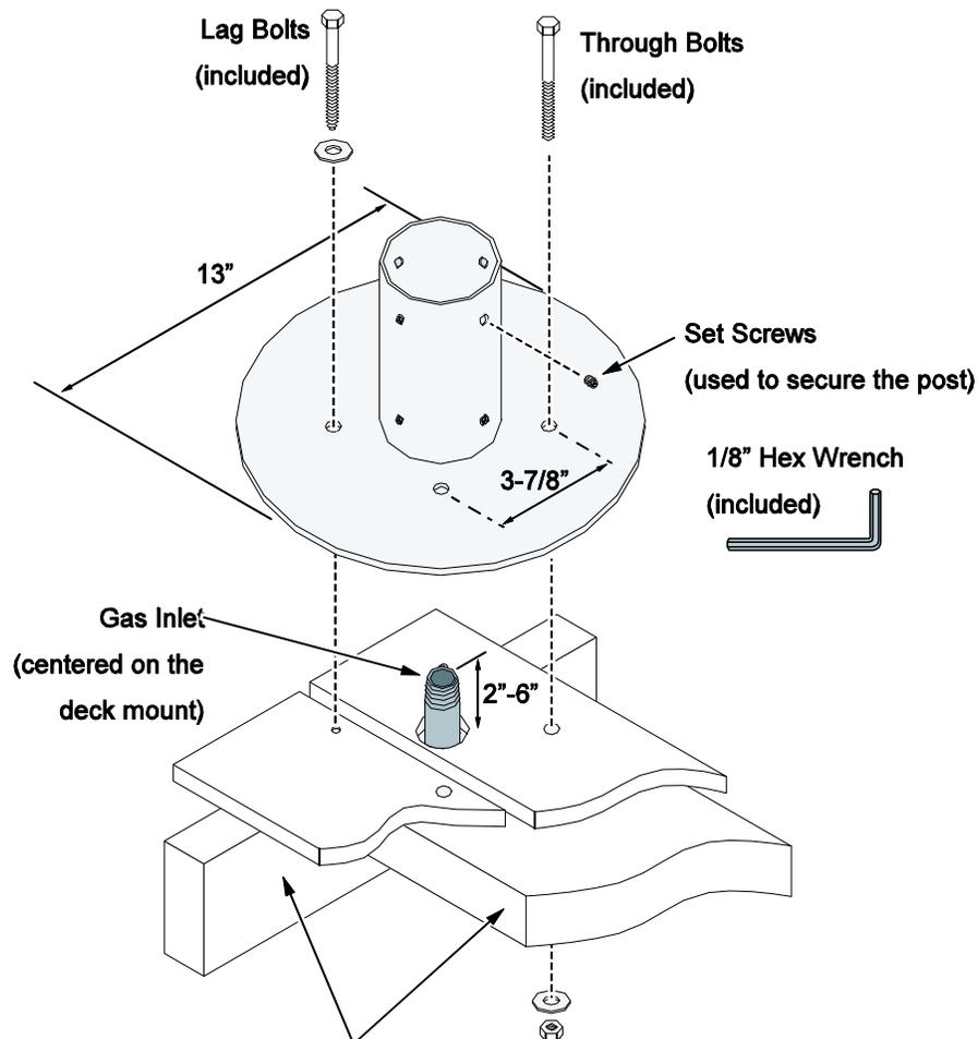
The post mount **must be secured to deck framing in four locations** (or other secure footing - the deck surface is not adequate for proper support).
